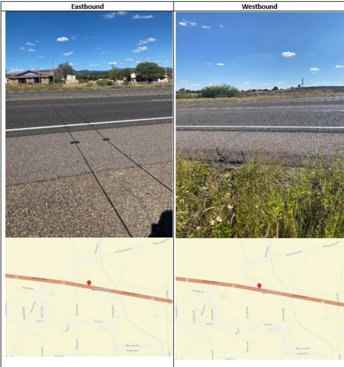
Figure 24. JAMAR Counter, East of Morales Road (Esri, HERE, Garmin, FAO, NOAA, USGS, OpenStreetMap contributors, and the GIS User Community, 2023)
