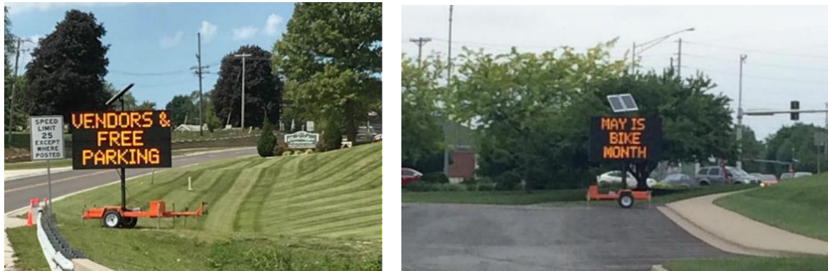
An LED dynamic message sign is a flexible ITS asset available for local governments to communicate information for special events or ongoing issues such as safety in small communities that do not have their own law enforcement. Images courtesy Mo-Kan.
